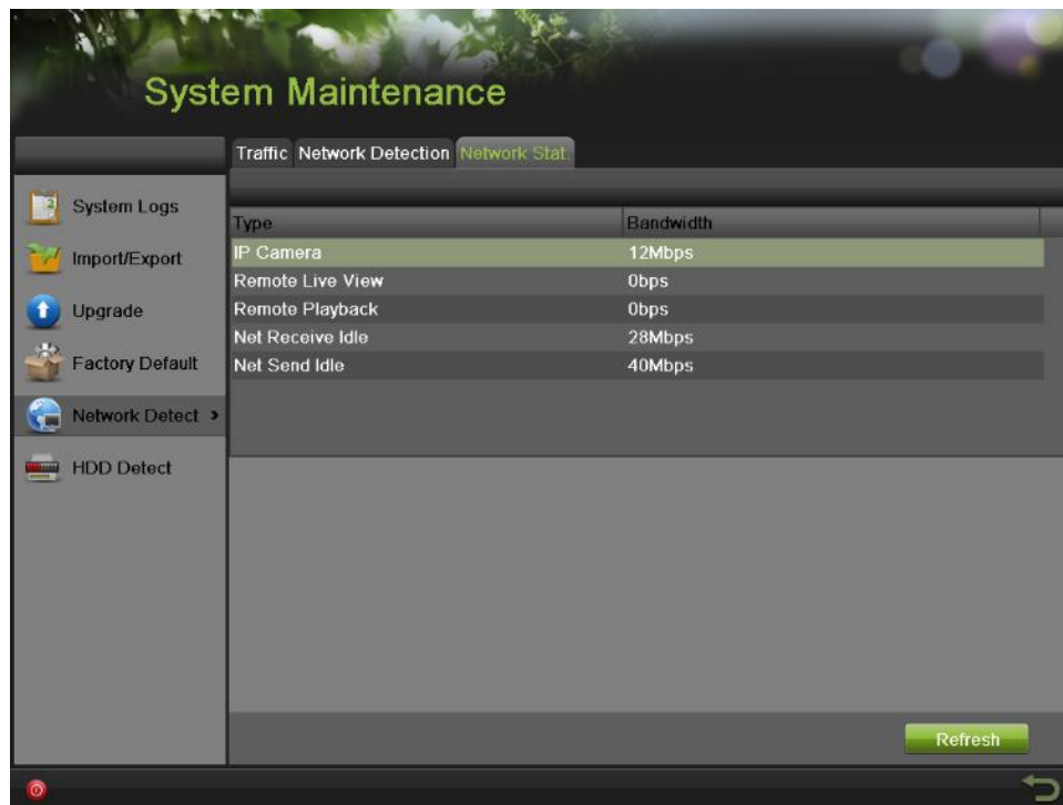
Figure 115 Network Stat. Interface
